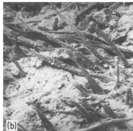
Figure 5 Fracture surfaces of oven dried Kinleith cellulose-cement composite (120 \times ). (a) Machine direction; and (b) cross direction.
