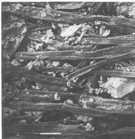
Figure 1 Kinleith cellulose fibres in cement matrix. Alignment of fibres is along the machine direction (120 X).
